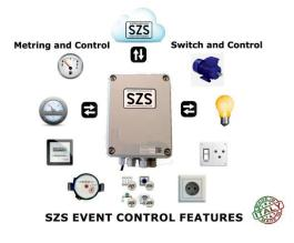
If for example the event that you want to control was the opening and closing of a passage now controlled locally by means of key access, remote control, badge card, simply by coupling one ShareZeroSpace device to the opening and closing command will be immediately possible to handle such passage, remotely from anywhere in the globe through the cloud.
